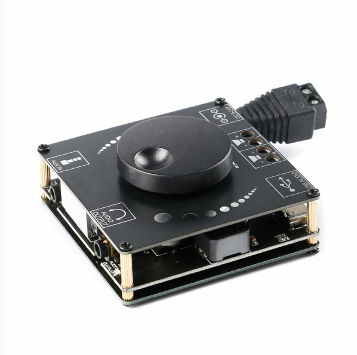
Image 4.1: Top view of the XY-AP50H amplifier board, showing the main components including the volume knob, power input, speaker terminals, AUX input, and USB port.
