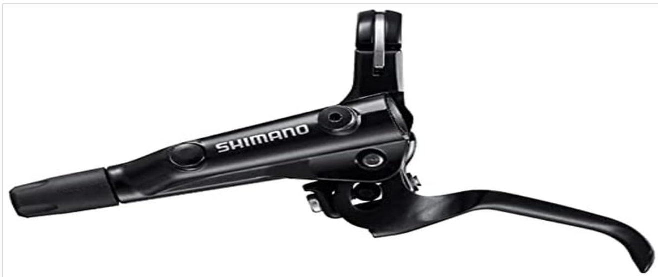
Figure 1: Shimano Deore BL-MT501 Left Hand Disc Brake Lever. This image shows the black aluminum lever body, the lever blade, and the clamp band mechanism for handlebar attachment.
