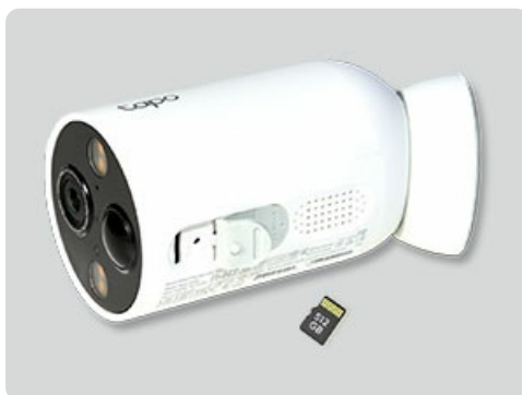
Figure 4.4: An illustration showing the location of the microSD card slot on the Tapo C425 camera.
