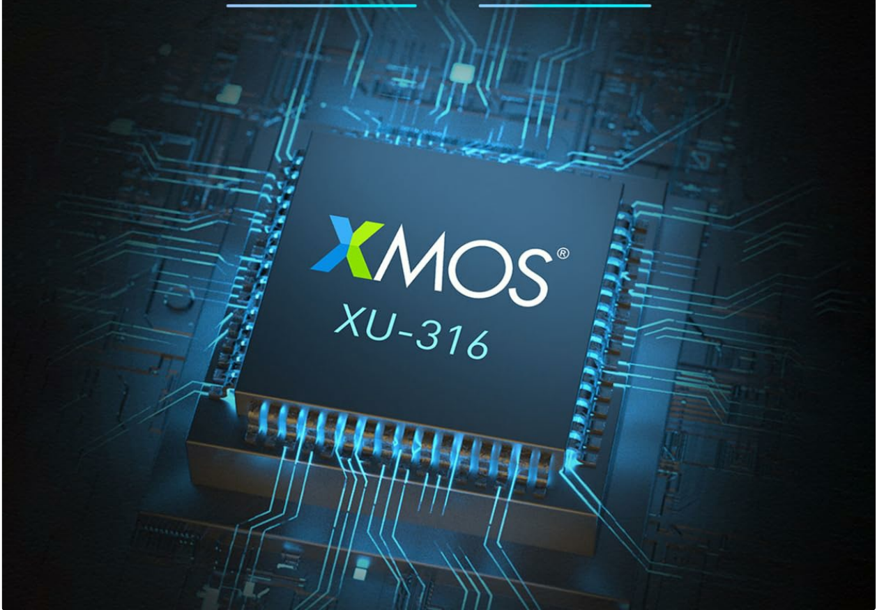
Figure 3.4: A detailed view of the XMOS XU-316 USB solution chip, emphasizing its support for DSD512 and PCM 32bit/768kHz.
