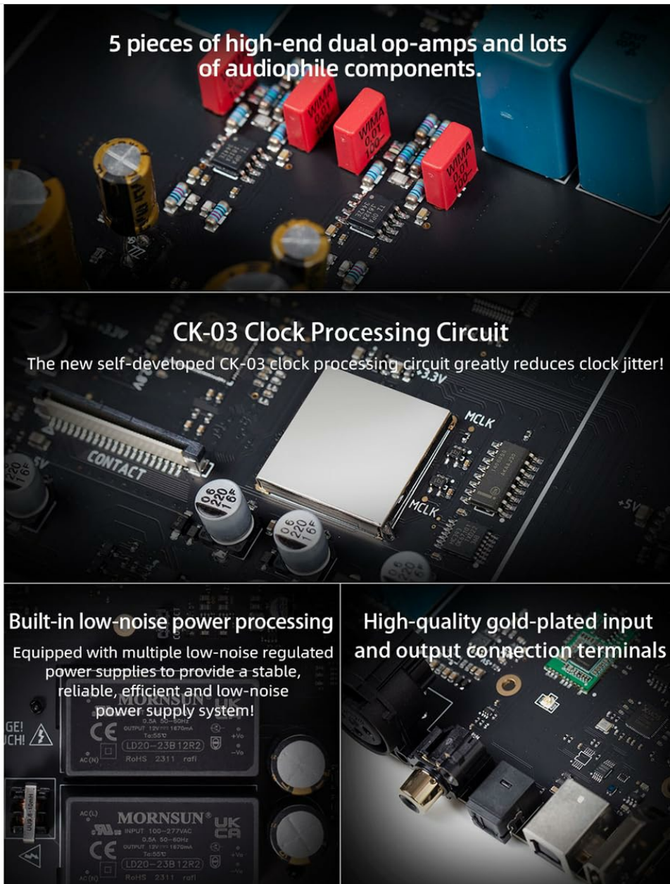
Figure 3.6: An internal view highlighting the 5 high-end dual op-amps, the CK-03 clock processing circuit, built-in low-noise power processing, and high-quality gold-plated input/output connection terminals.
