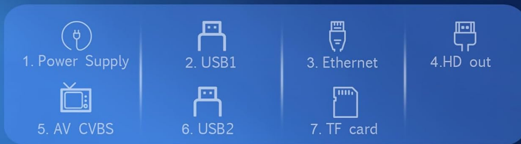
Image: Diagram illustrating the various ports and their functions on the Sawgmore Q1 TV Box.
