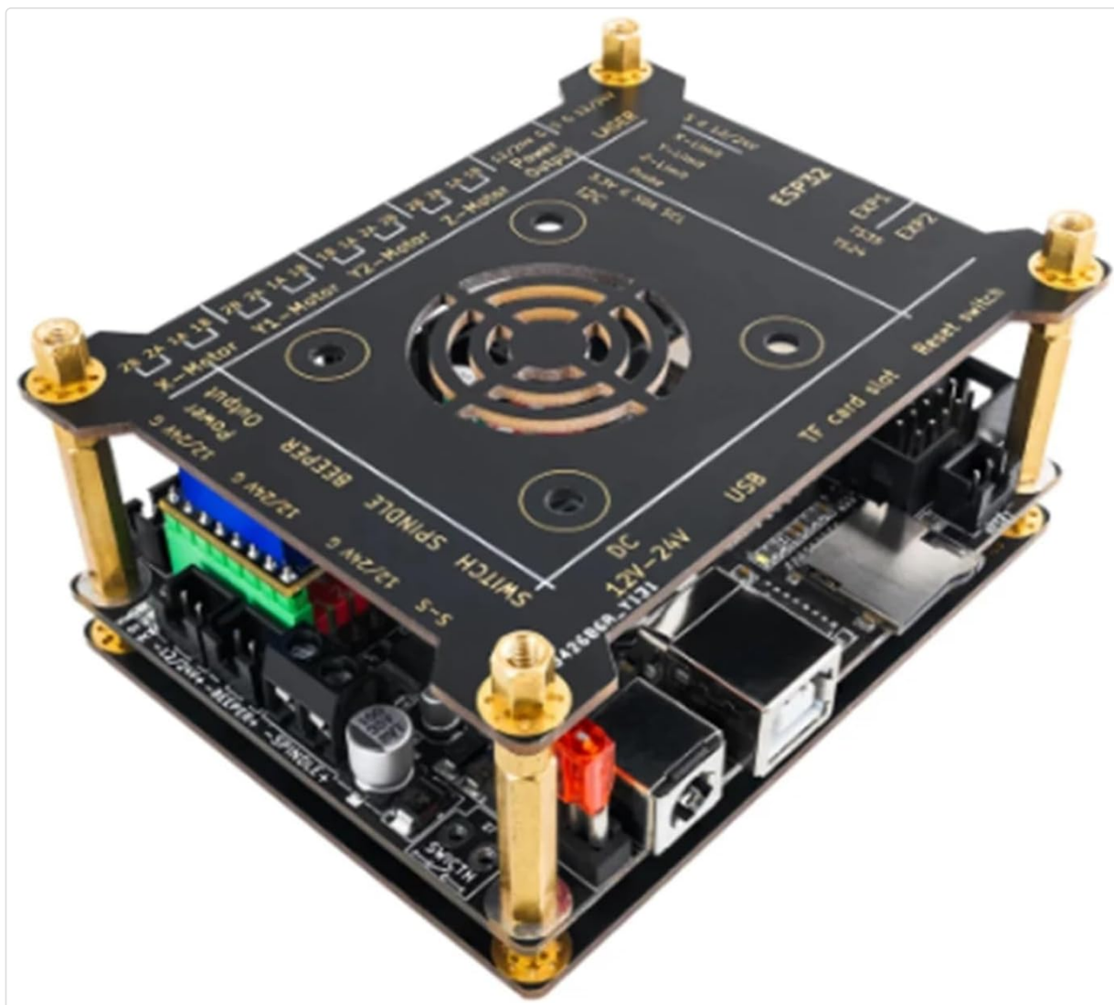
Image 5.1: The MKS DLC32 V2.1 board housed within a protective casing, demonstrating an option for enhanced durability.
