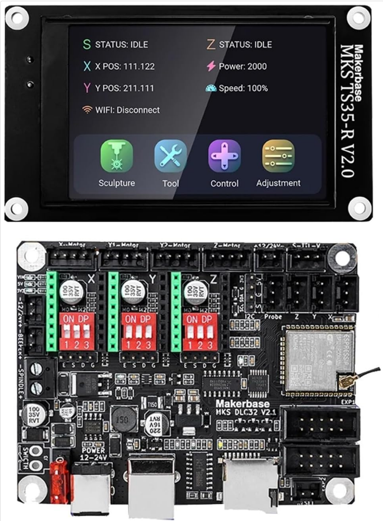
Image 3.1: Visual representation of the MKS DLC32 V2.1 board and its connection points, including the TS35-R display.
