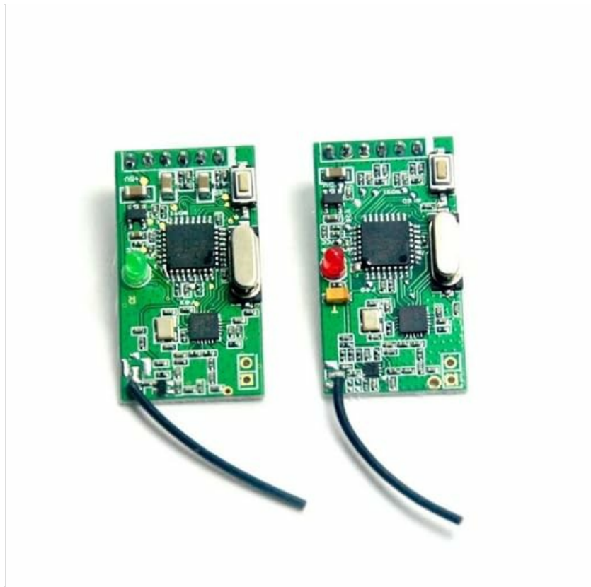
Figure 2.1: Ubden 2.4G NRF 24L 01 Wireless Digital Audio Transceiver Modules (Transmitter and Receiver).
