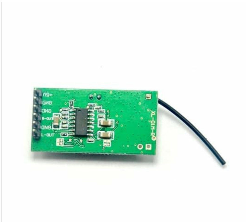
Figure 2.2: Rear view of a single NRF 24L 01 module, highlighting connection pins.
