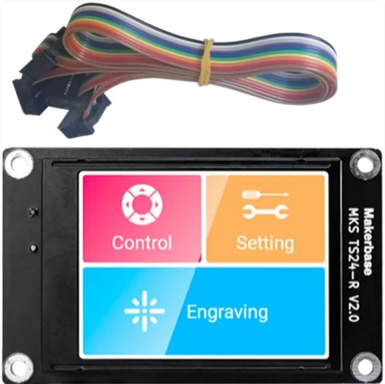
Figure 3.1: The MKS TS24-R V2.0 display unit and a typical ribbon cable for connection to the control board.
