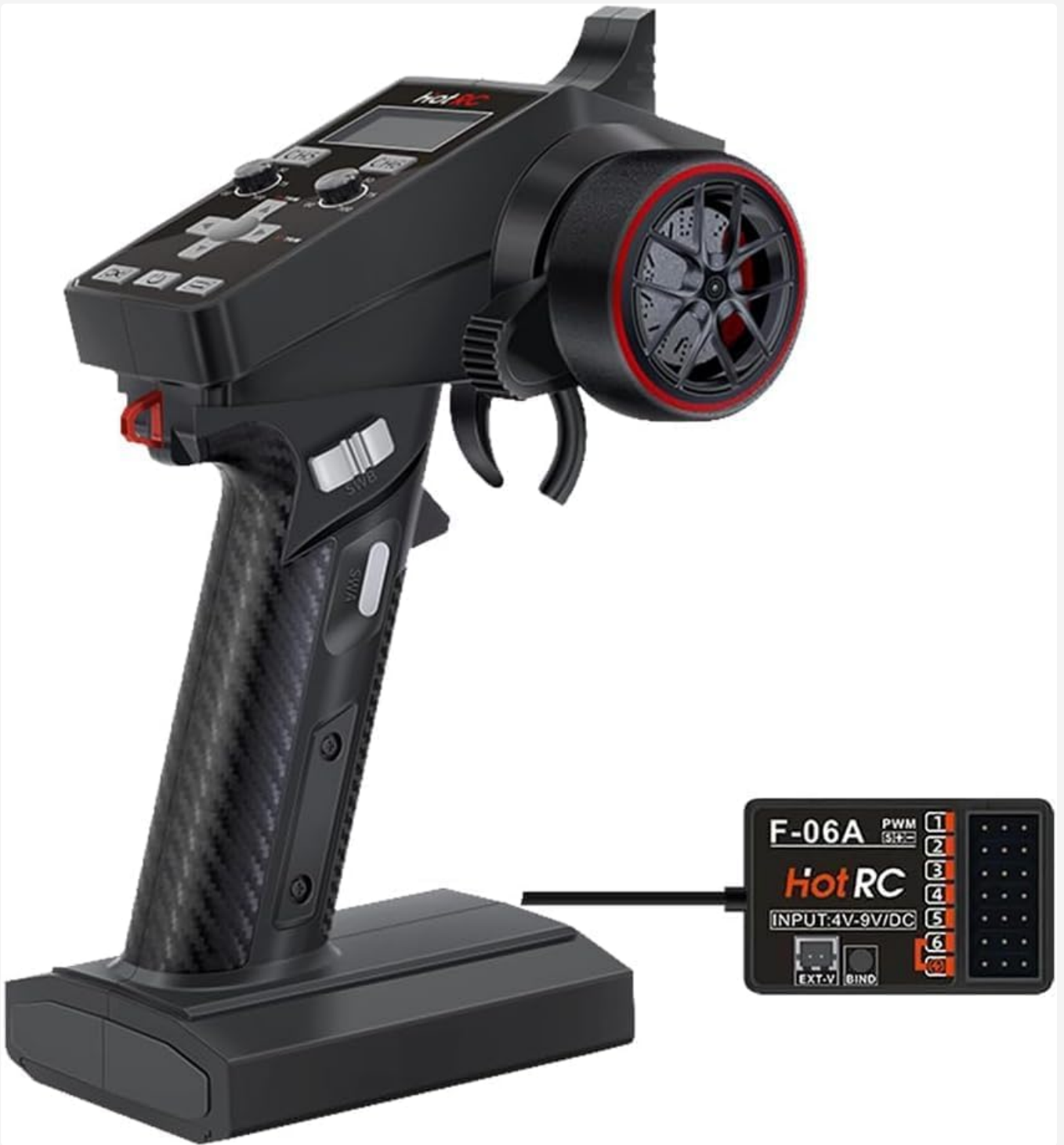
Figure 1: The HOTRC CT-6A 2.4GHz 6-Channel RC Transmitter and its accompanying F-06A receiver. The transmitter features a pistol grip design with a steering wheel for intuitive control, while the receiver provides 6 PWM channels and a bind button.
