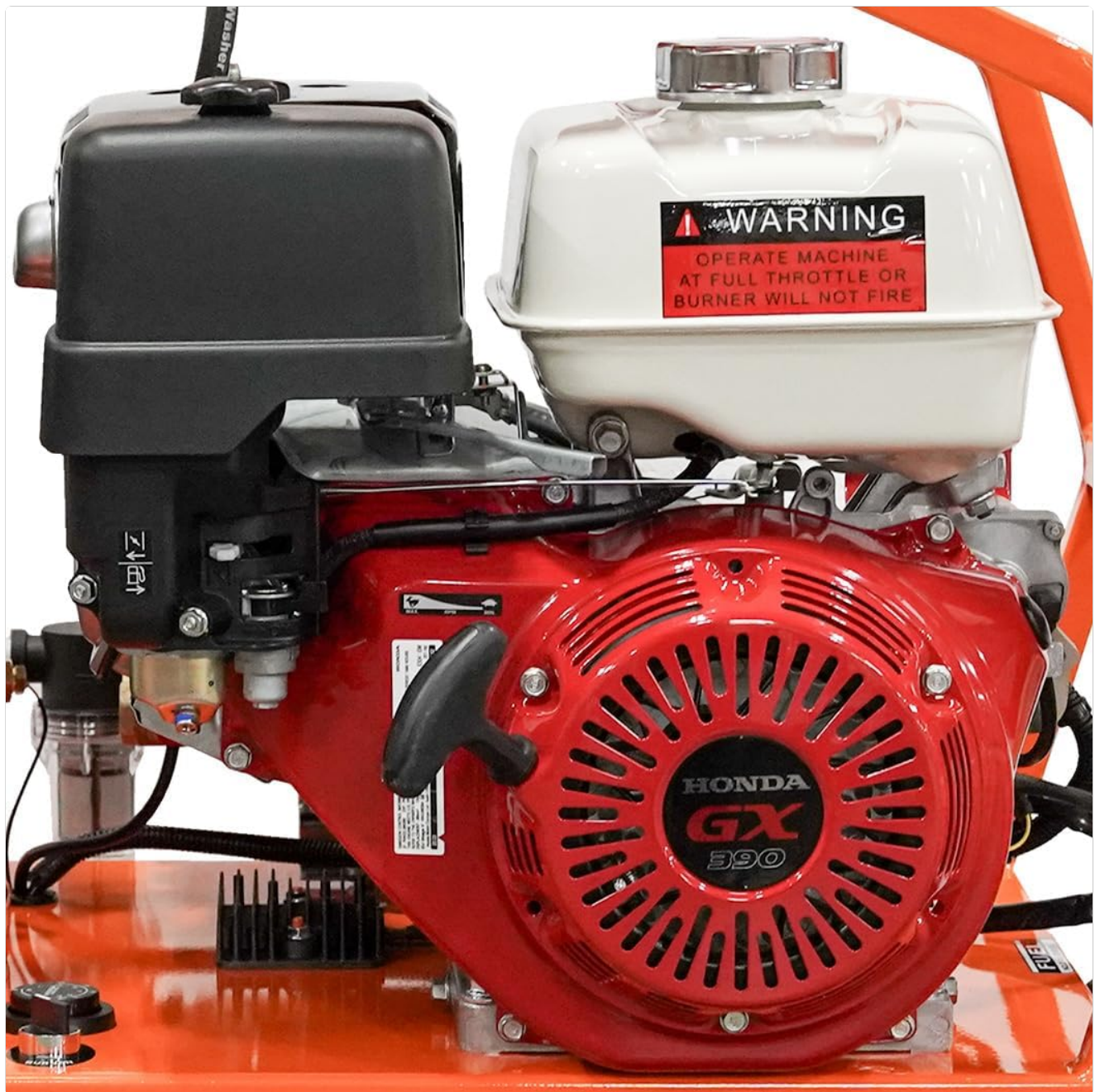
Figure 4.1: Detail of the Honda GX390 engine, indicating fuel and oil points.
