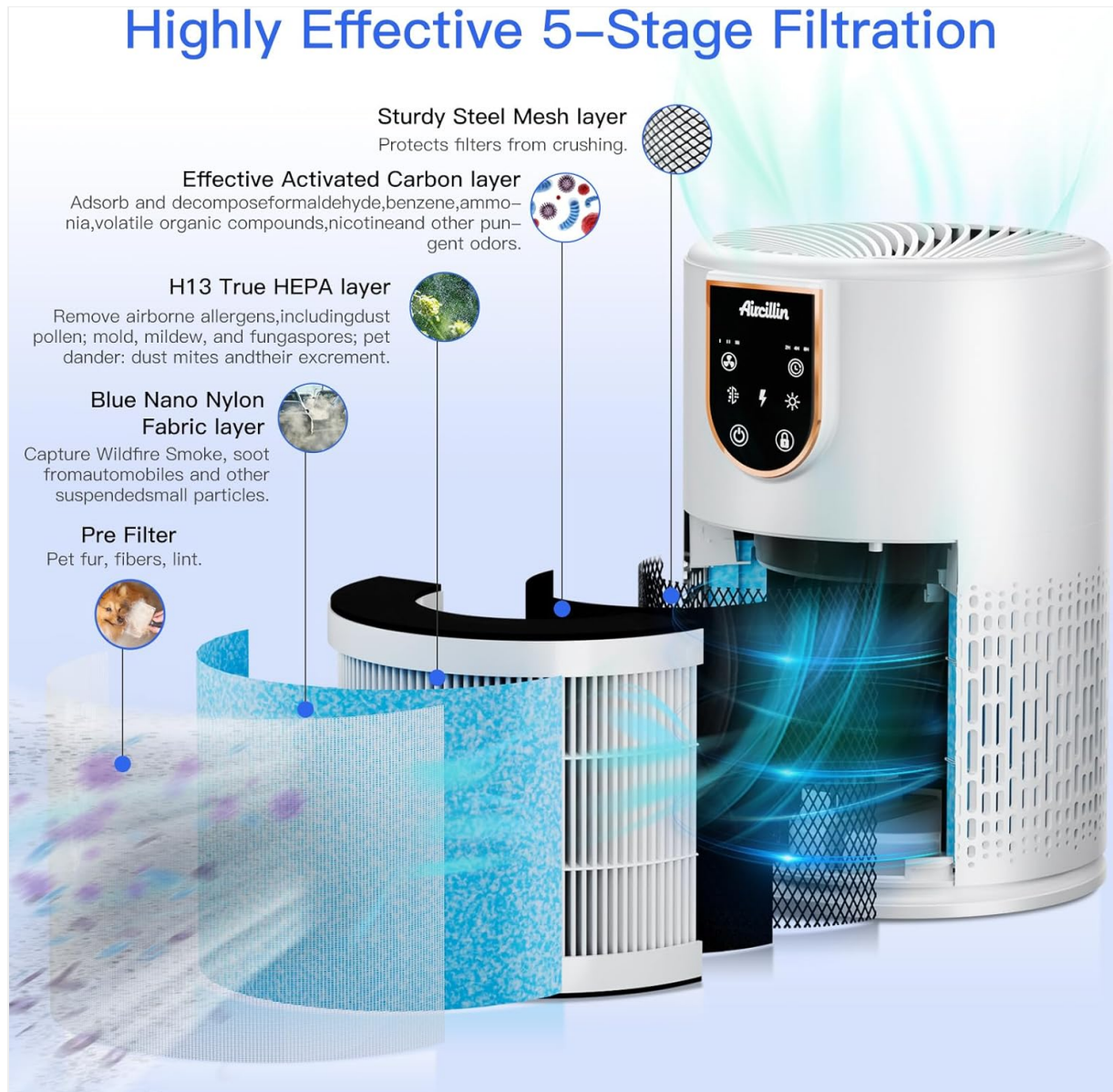
Image 3.1: Exploded view of the Aircillin AP0801 Air Purifier's 5-stage filtration system, detailing the Sturdy Steel Mesh layer, Effective Activated Carbon layer, H13 True HEPA layer, Blue Nano Nylon Fabric layer, and Pre-Filter.
