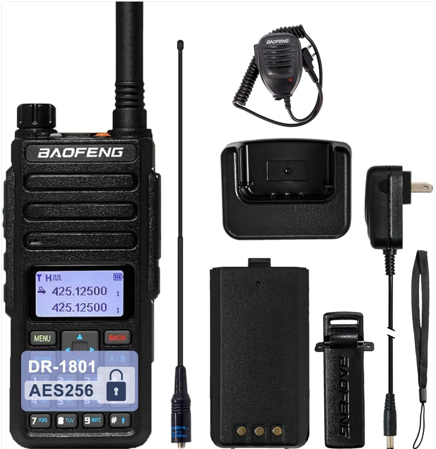
Figure 3.1: Contents of the BAOFENG DR-1801 package, including the radio, battery, antennas, charger, belt clip, hand strap, and speaker microphone.
