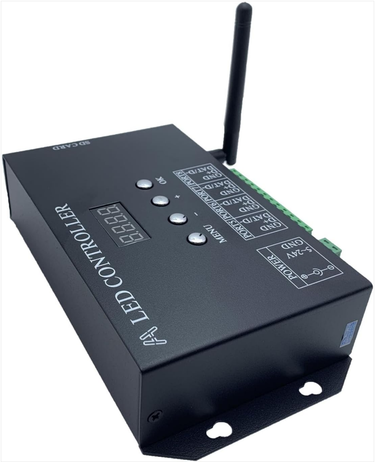
Figure 1: Top view of the H807SB controller, showing power input, output ports (DAT/D, GND), and control buttons (OK, MENU).
