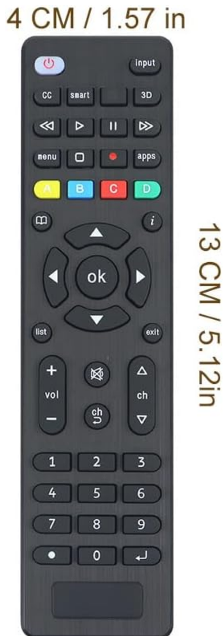
Figure 5: Pilotage Universal Remote Control with dimensions.
