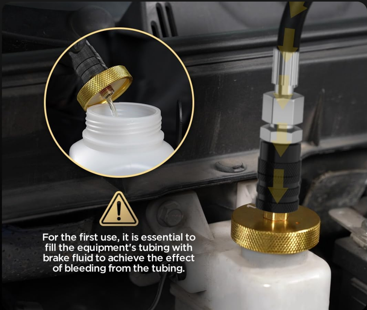
Figure 4: Illustration of the air-free filling process for the equipment's tubing.
