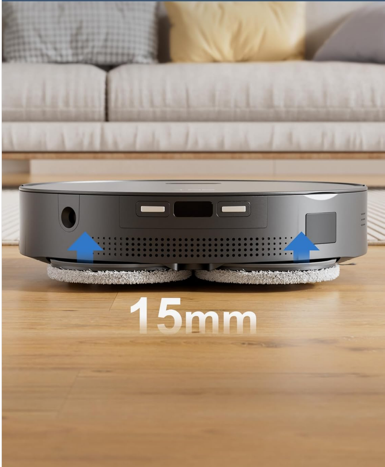
Figure 7: The automatic 15mm mop lifting feature protects carpets during mopping cycles.
