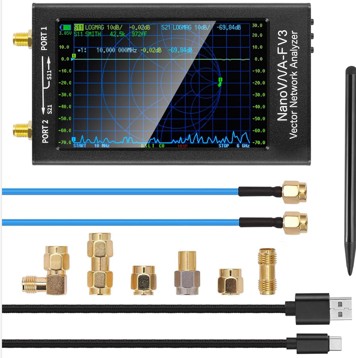
Figure 1.1: The NanoVNA-F V3 Vector Network Analyzer and its included accessories, including SMA cables, adapters, and a stylus.
