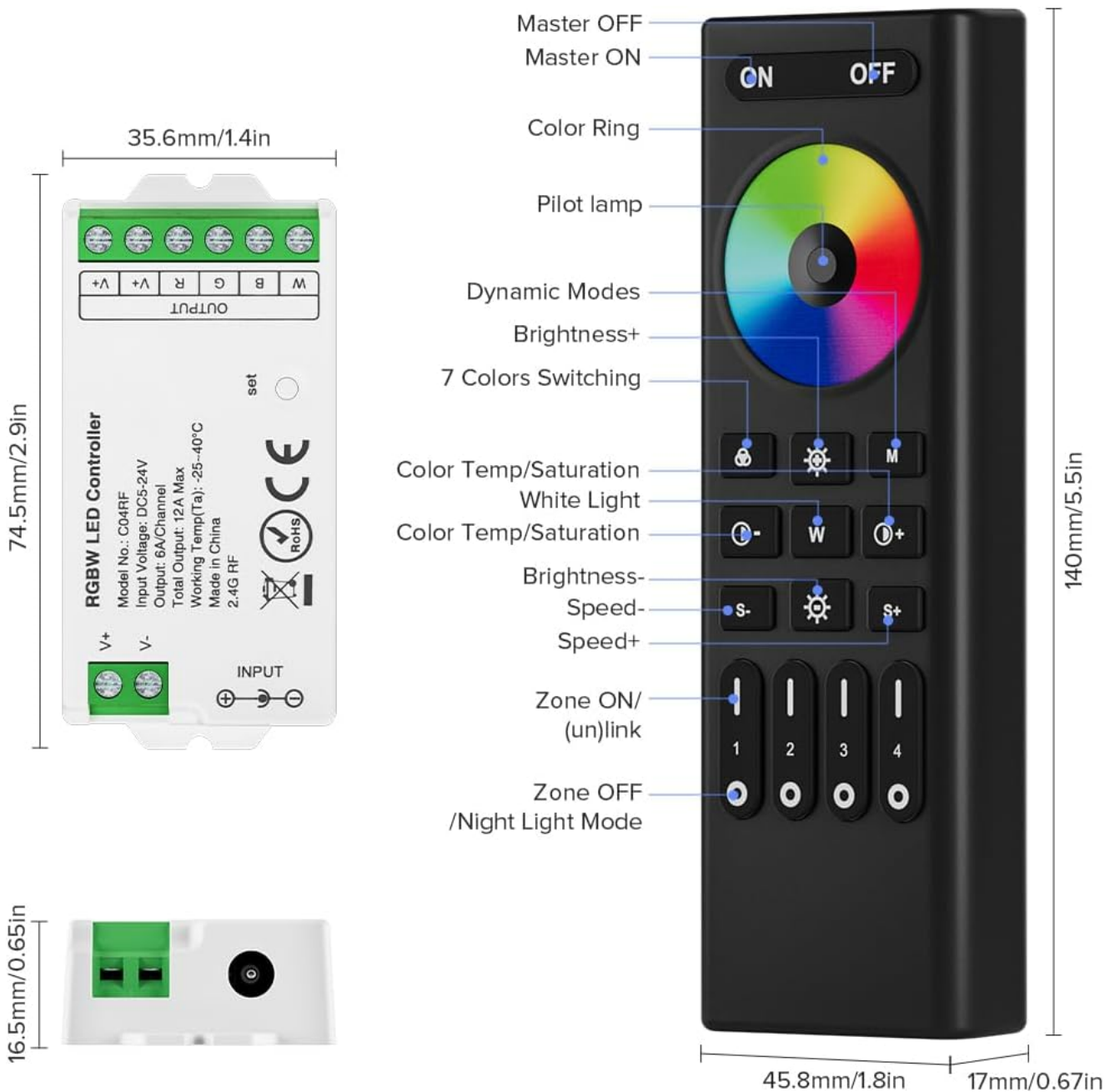
Image 3.1: Diagram illustrating the buttons and functions of the RC03RFB remote control and the C04RF controller.
