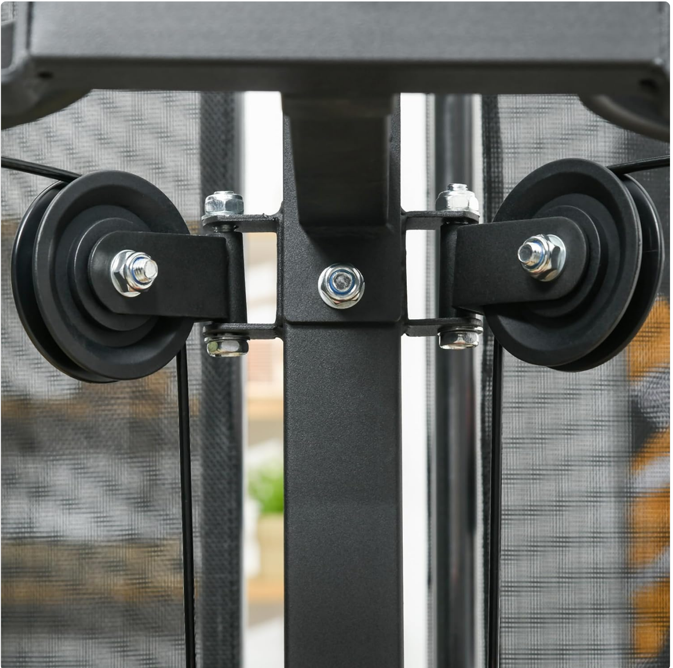
Figure 3.2: Cable and pulley system detail
