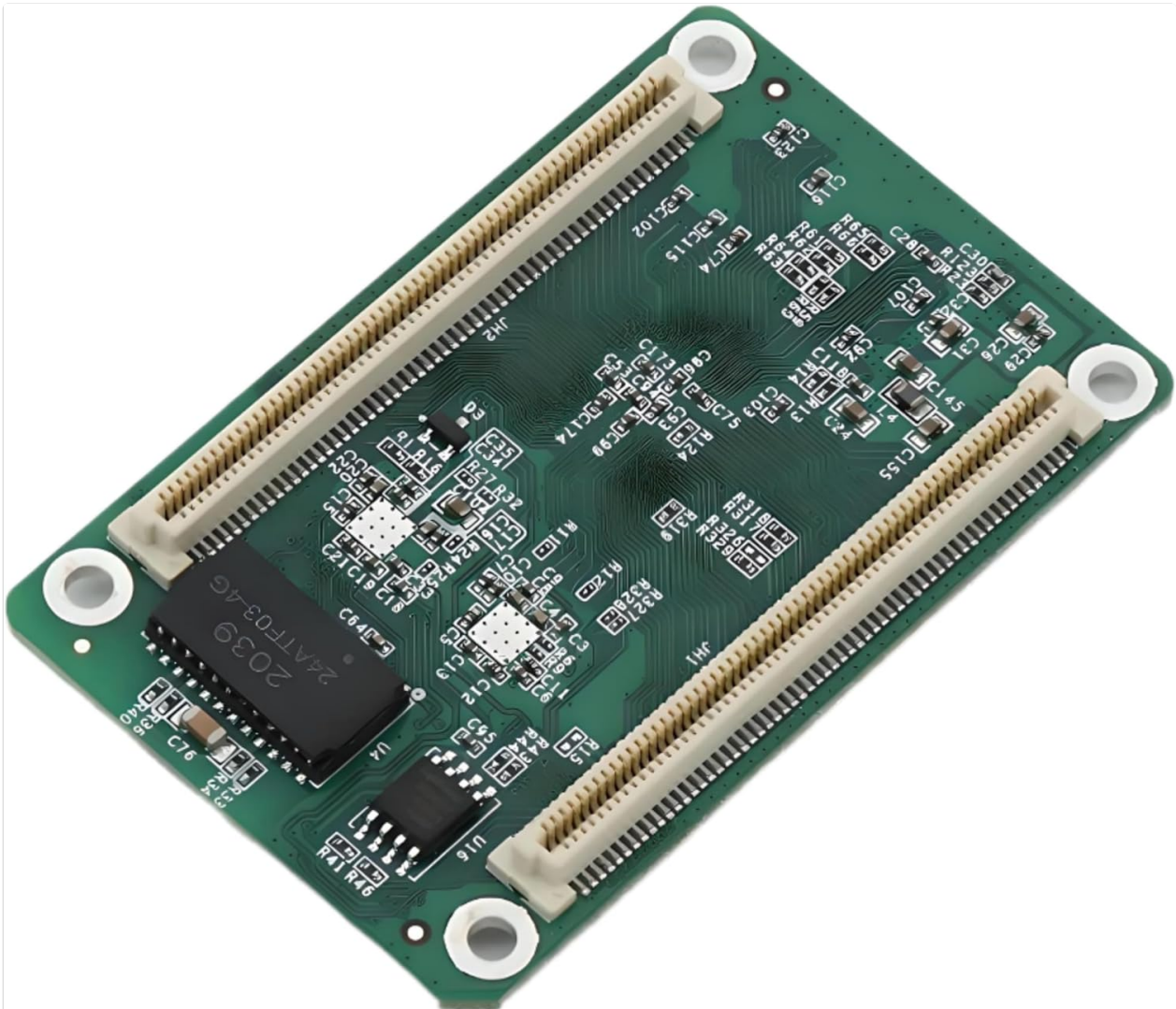
Figure 2: Back view of the NovaStar A5s Plus LED Receiving Card, highlighting the multiple HUB75E connectors for LED module data input/output.
