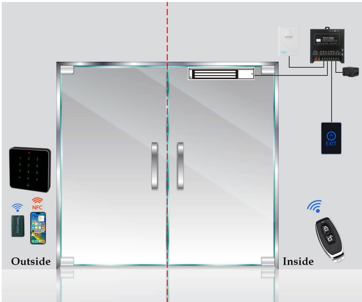
Figure 3.1: An overview diagram illustrating the typical placement of the keypad, magnetic lock, power supply, exit button, doorbell, and remote control receiver relative to a door.
