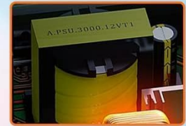
High Frequency Transformers
