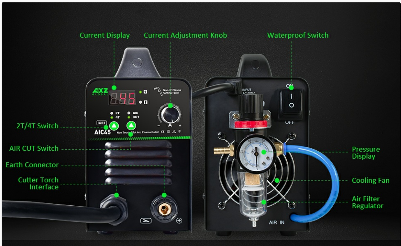
Image 5.1: Front and rear panel connections and controls.
