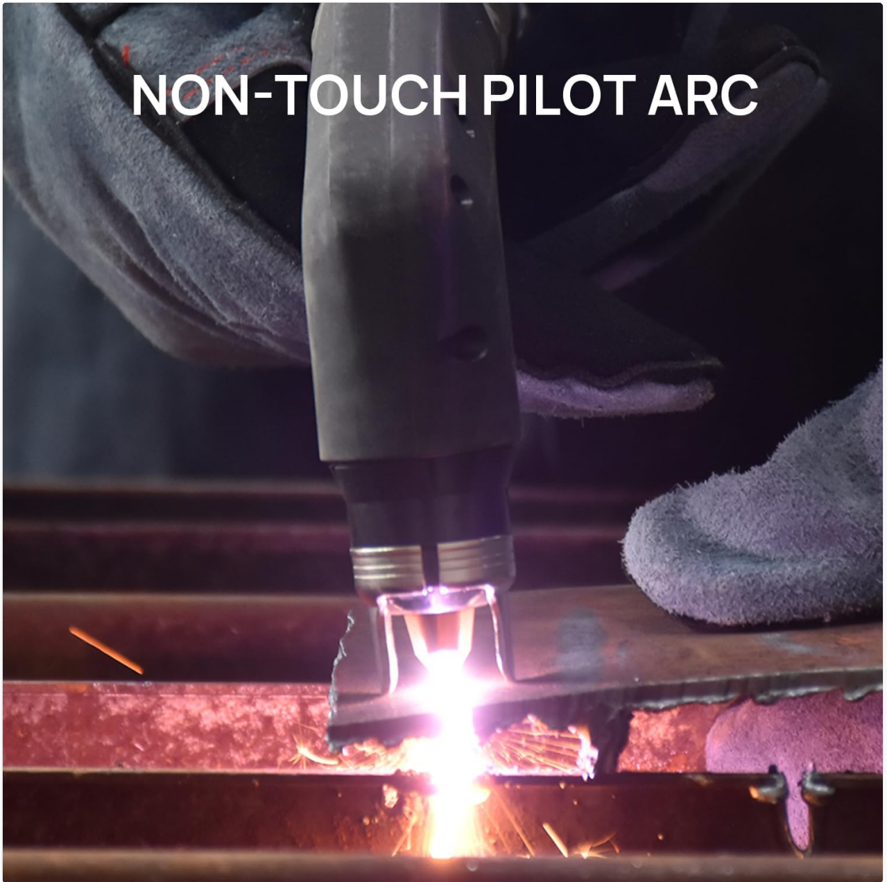
Image 4.2: Non-touch pilot arc in action.
