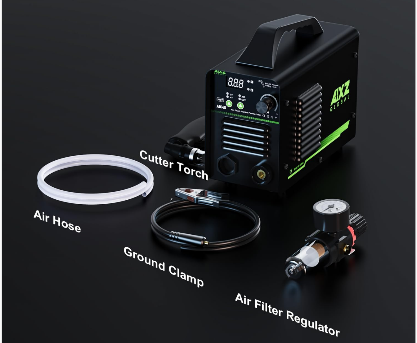
Image 3.1: Included plasma cutter equipment components.
