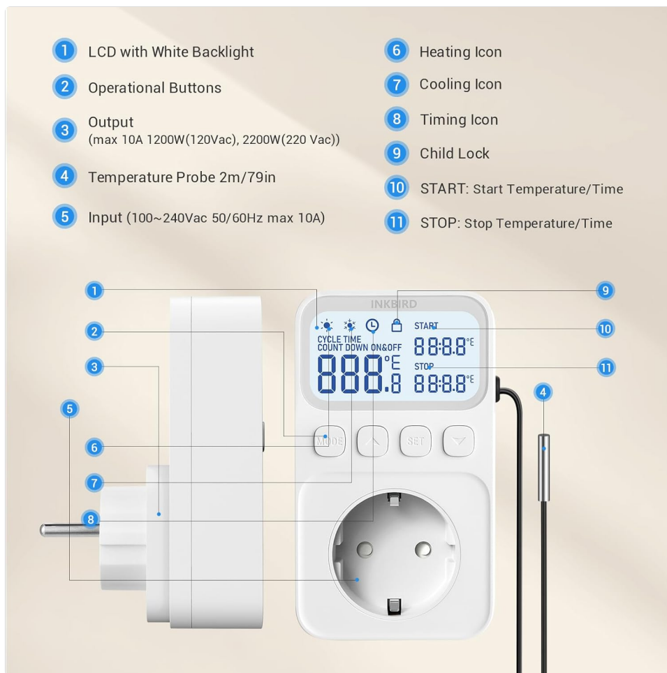
Image: Detailed diagram of the Inkbird ITC-C216T thermostat with labeled components.
