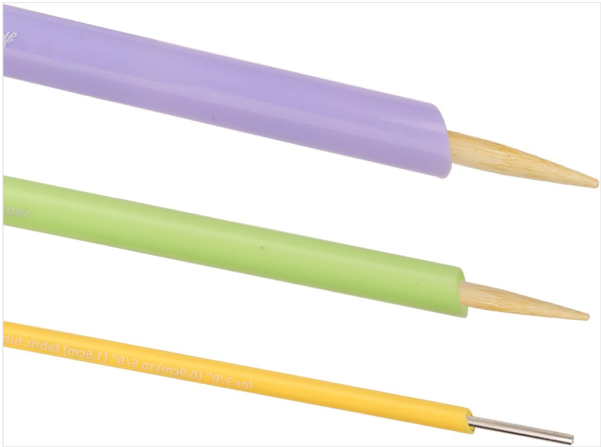
Figure 2: A close-up view of the three fabric tube turners, highlighting their distinct sizes and the pointed wooden sticks used for pushing the fabric.
