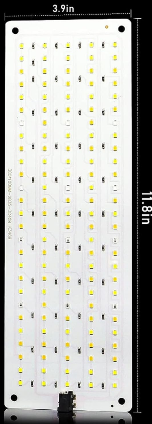
Image: Detailed diagram of the full spectrum grow light, indicating the distribution of different LED types (Cold White, Warm White, Red) and a spectral graph illustrating the light output across various wavelengths. Dimensions of the light are also shown.
