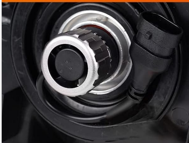
Figure 5.2: No External Ballast Required for SEALIGHT Bulbs
