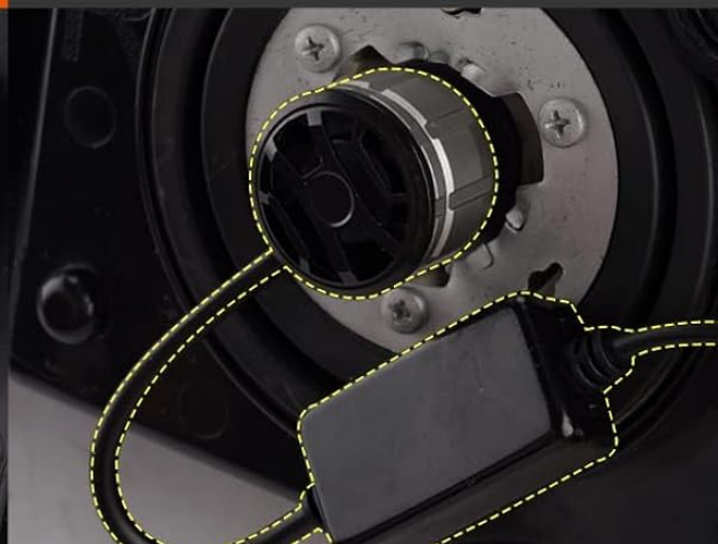
Figure 5.2: No External Ballast Required for SEALIGHT Bulbs
