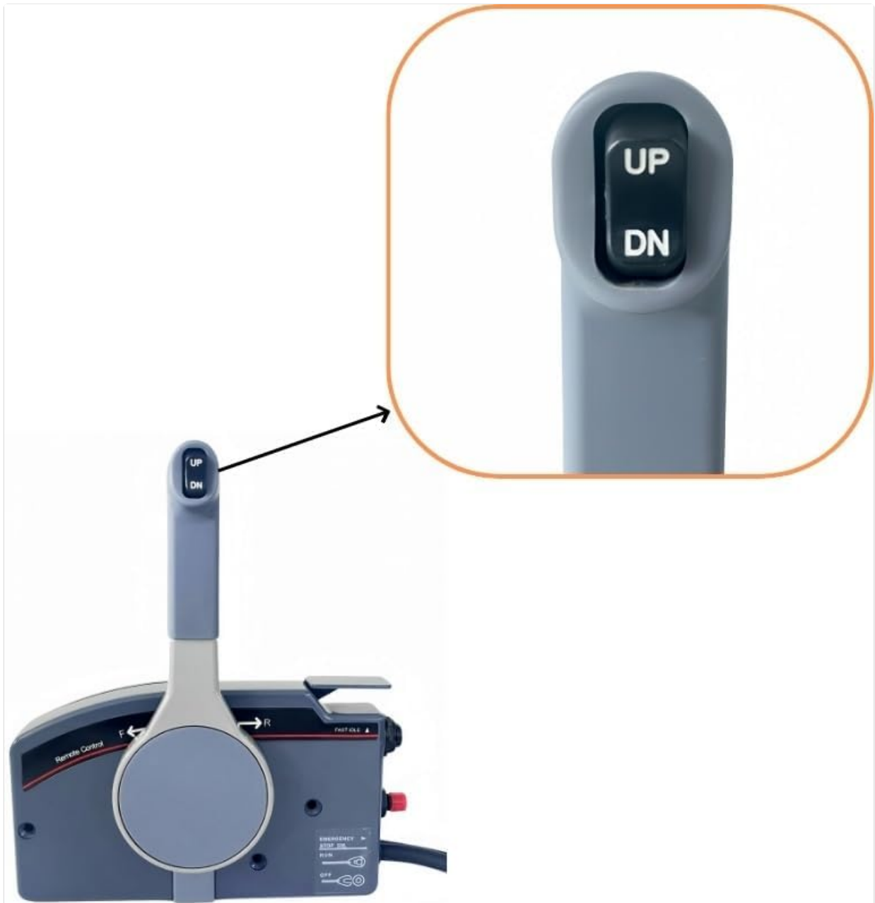
Figure 4.2: Detail of the UP and DN buttons for trim and tilt adjustment.
