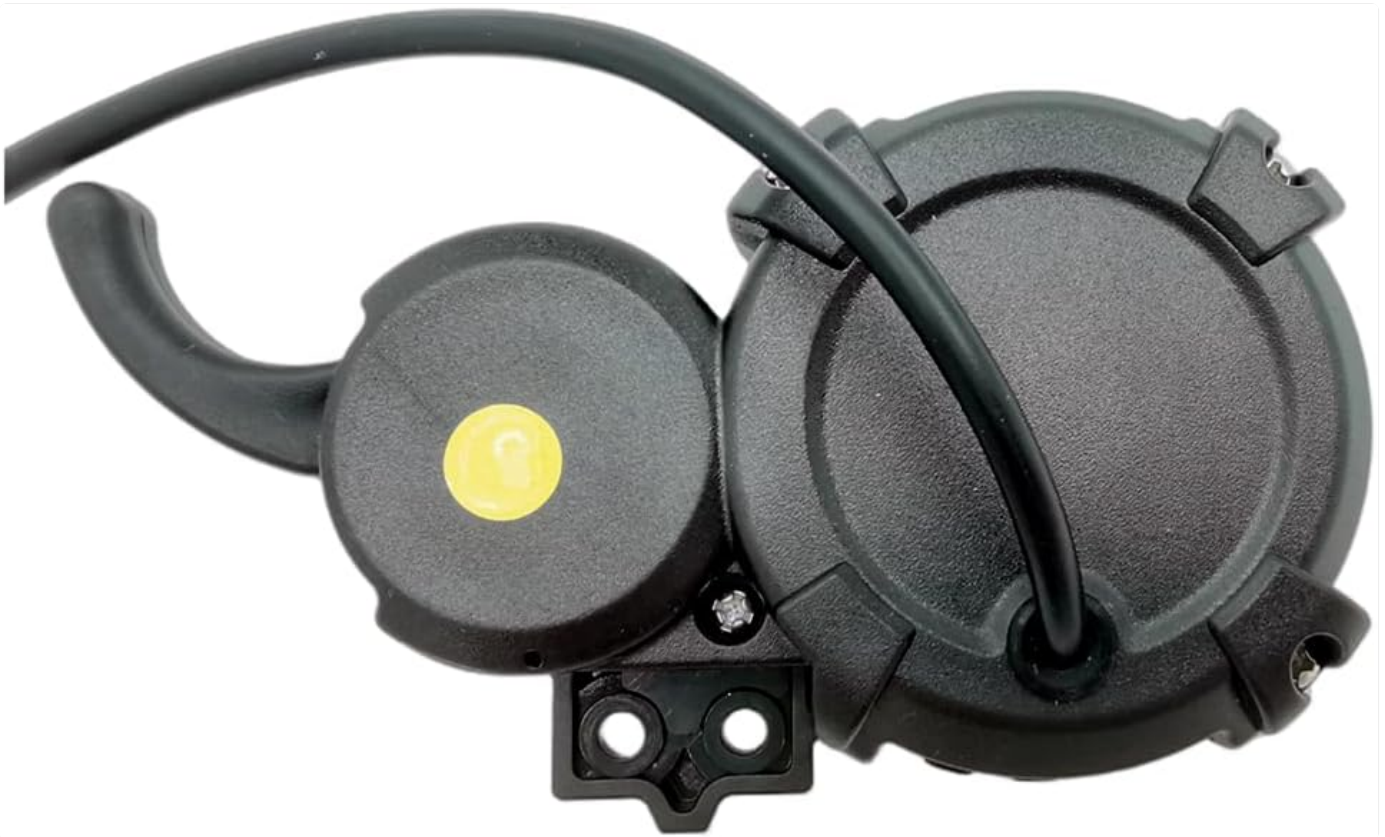
Figure 3: Rear view of the EY3 display and throttle assembly, showing mounting points and cable routing.
