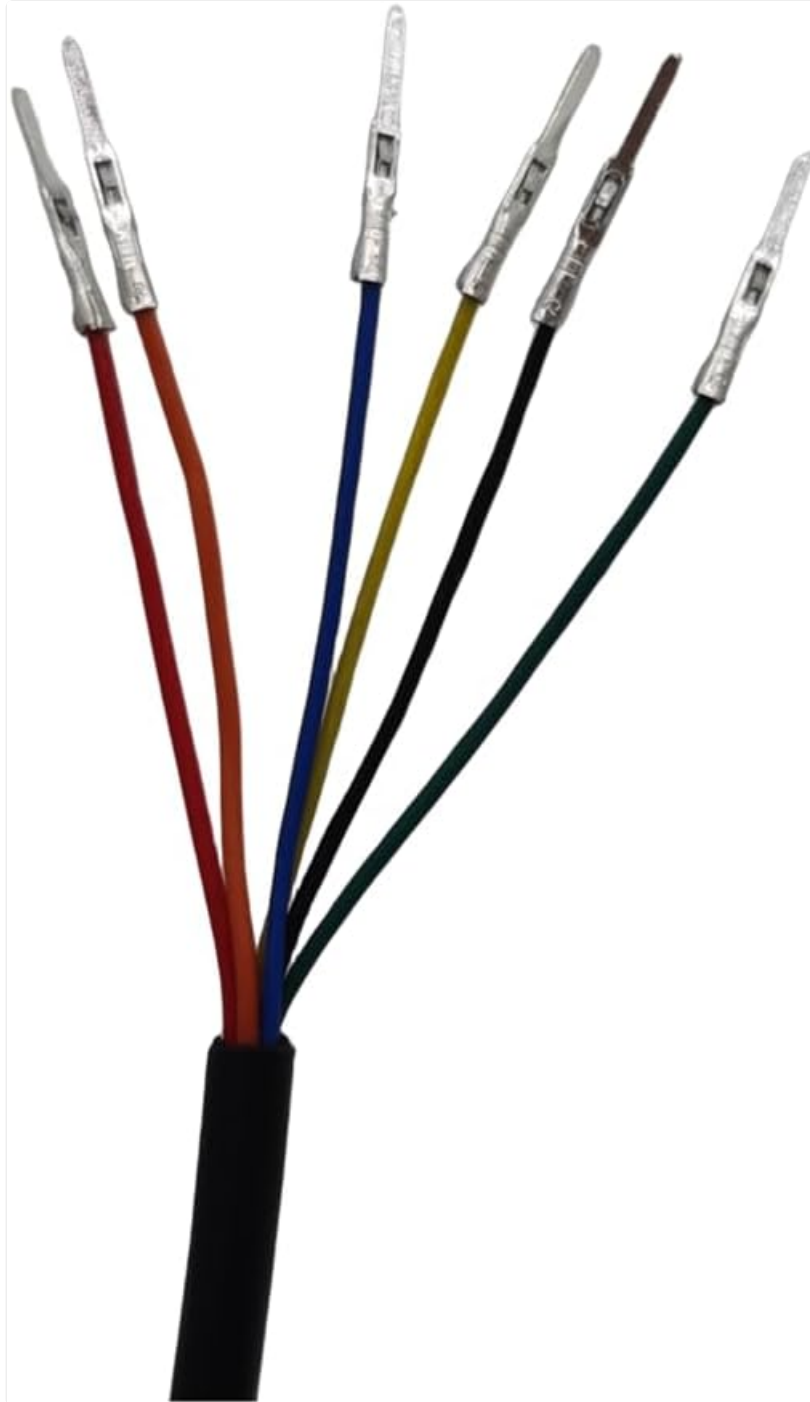
Figure 2: Close-up view of the multi-colored wiring harness for connecting the EY3 display to the scooter's electrical system.
