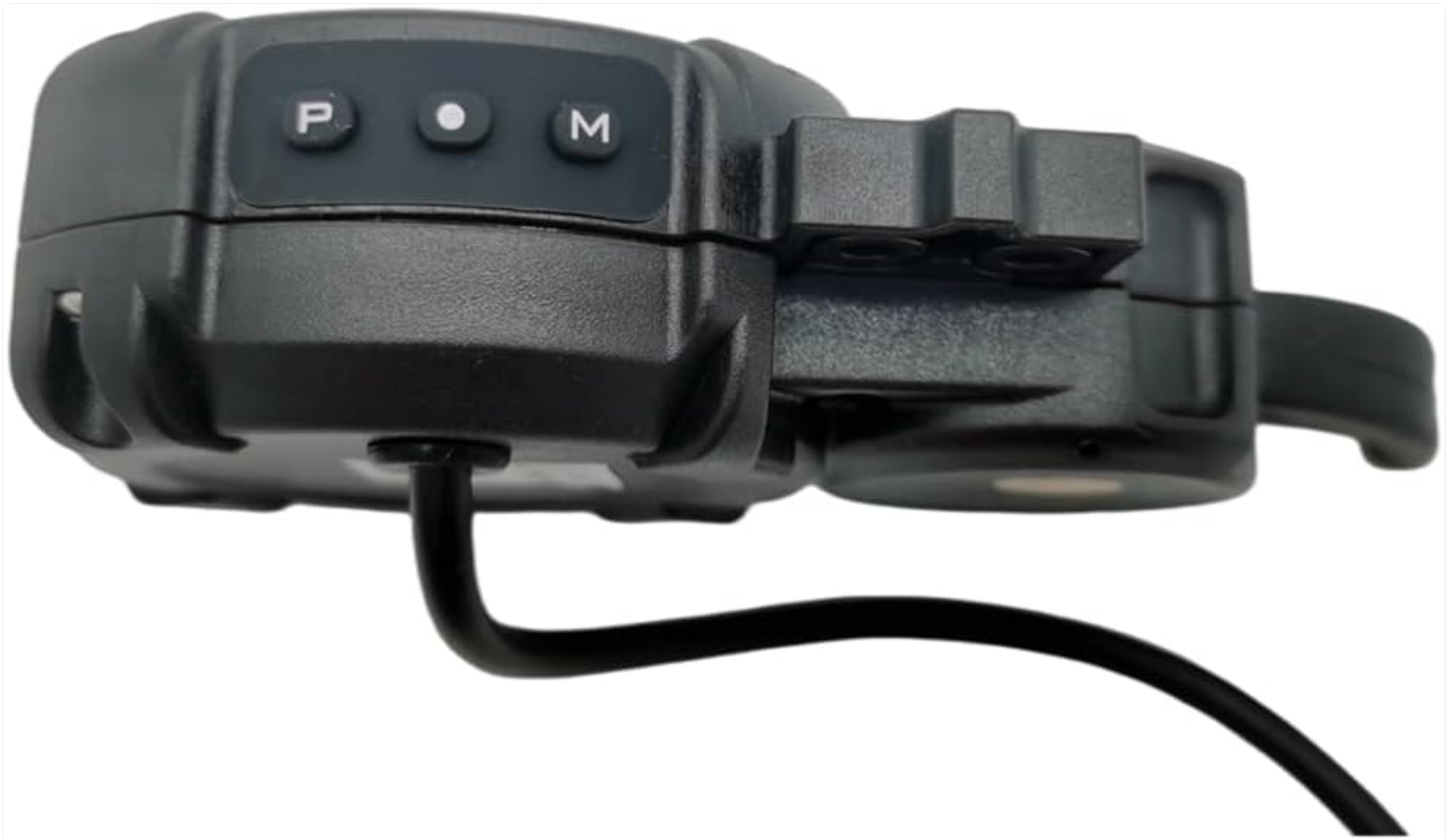
Figure 4: Side view of the EY3 display, highlighting the 'P' (Program) and 'M' (Mode) buttons used for menu navigation and setting adjustments.
