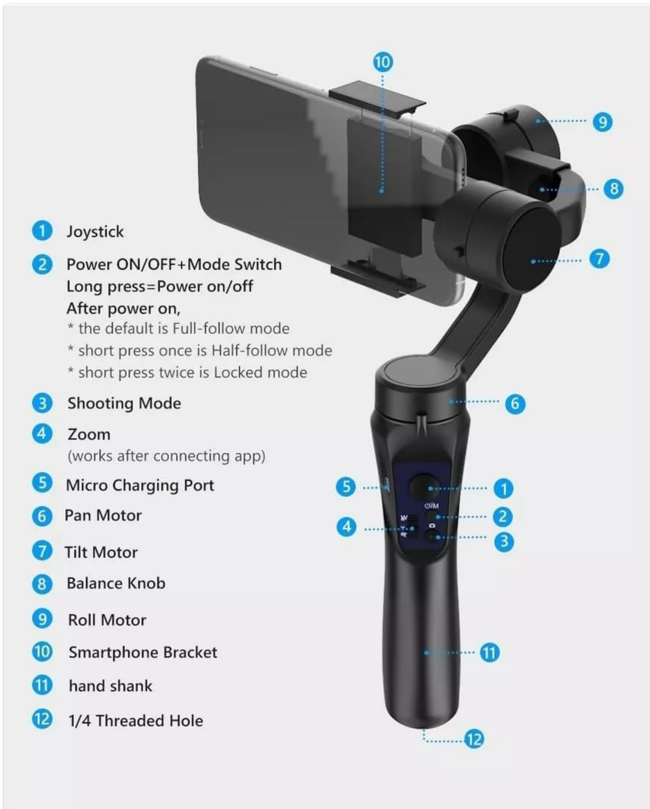
Figure 1: Axnen F6 Gimbal Stabilizer Parts Diagram
