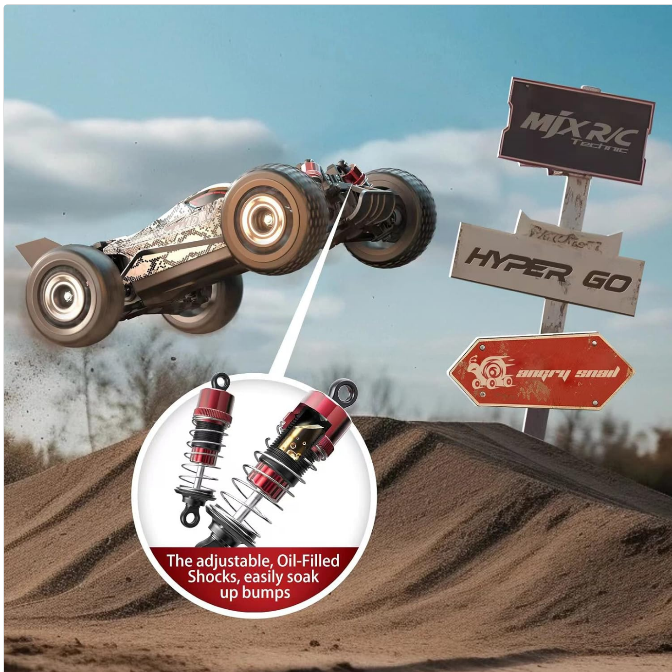
Image: The HYPER GO H16PL Buggy mid-air over a dirt mound, showcasing its adjustable, oil-filled shocks designed to absorb impacts during off-road driving. The image emphasizes the buggy's capability for dynamic terrain navigation.
