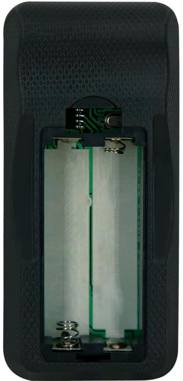
Figure 4: This remote control is designed for AAA batteries, offering longer durability compared to older coin battery designs.
