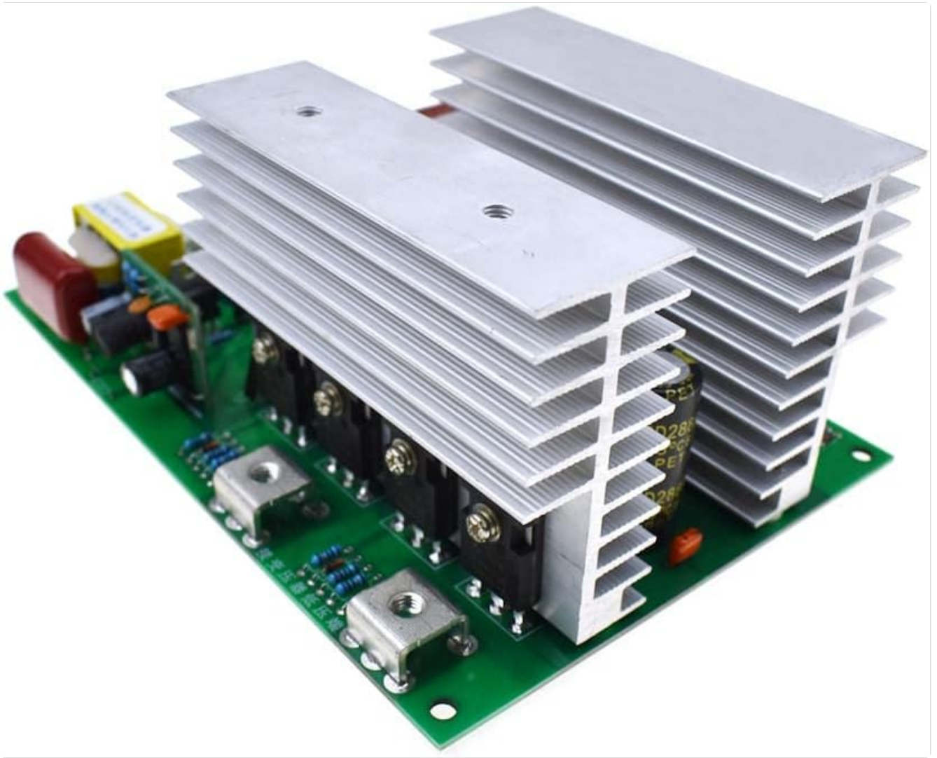
Figure 3.3: A detailed perspective showing the robust heatsinks and critical power components mounted on the motherboard, essential for thermal management.
