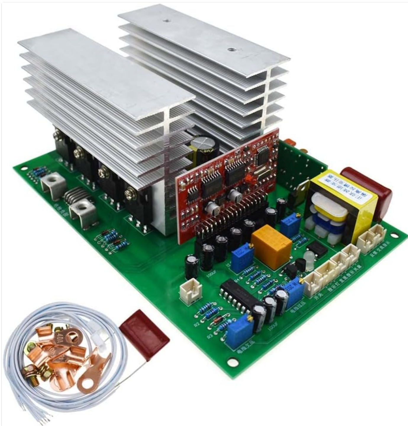
Figure 3.1: Overall view of the Reland Sun Pure Sine Wave Inverter Motherboard (12V1000W) along with accessory wiring and a capacitor.
