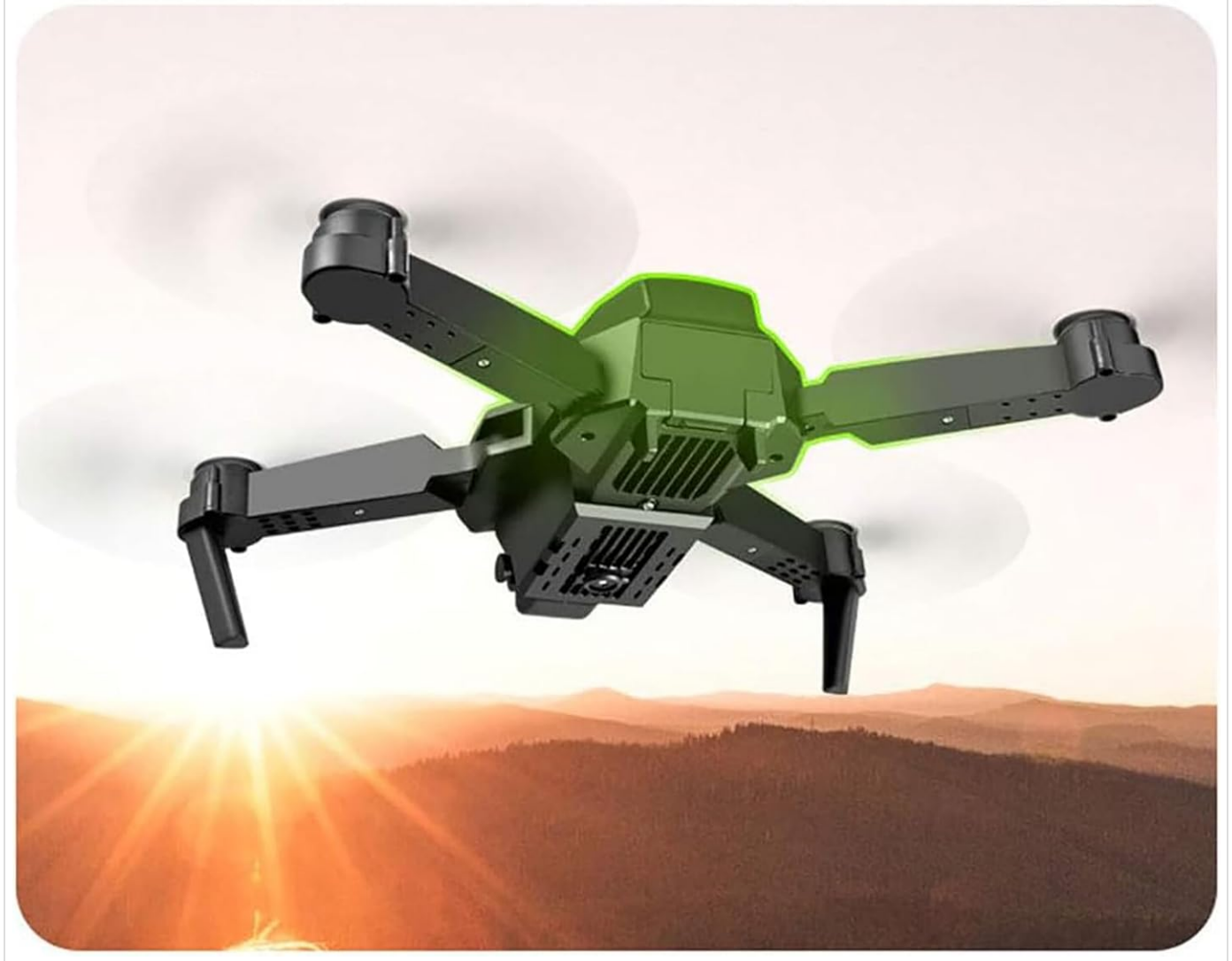
Image 4.1: The UNbit E88 Pro drone in flight, illustrating its 15-minute battery life with the equipped 3.7V 1800mAh battery.
