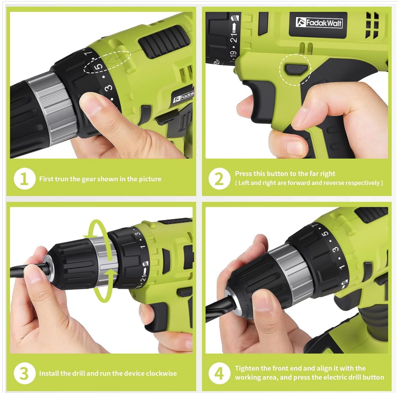
Figure 4.1: Bit Installation Steps
