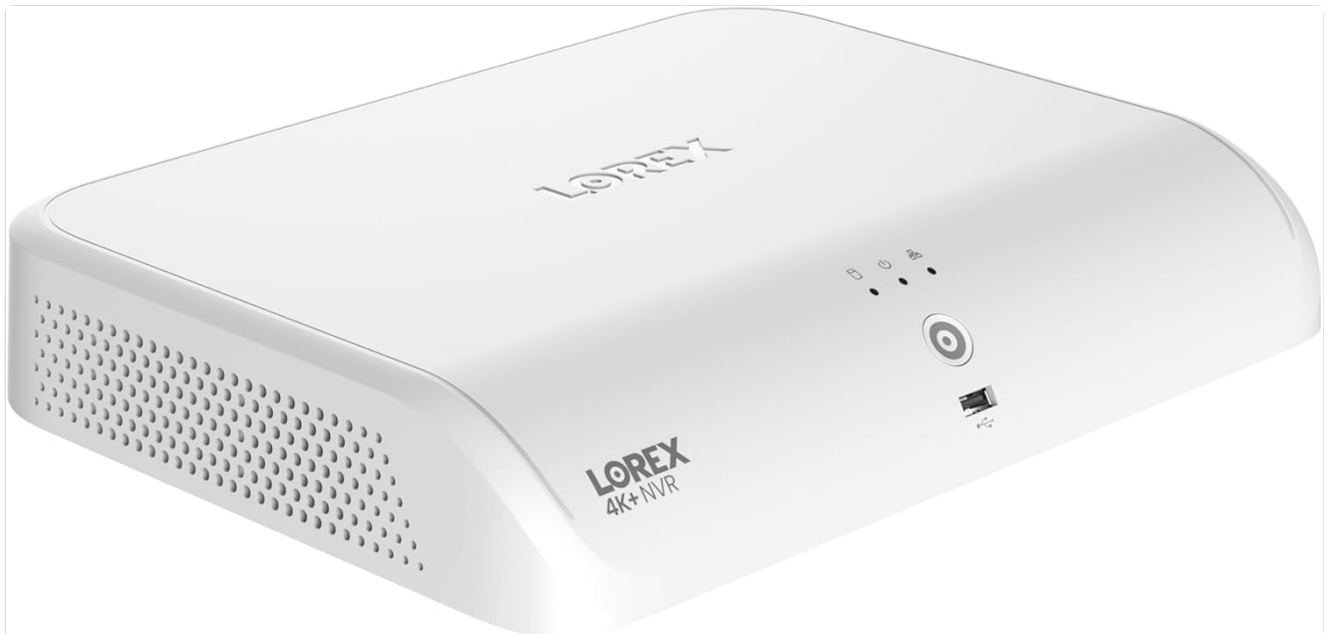
Figure 2.1: Front view of the Lorex 4K+ NVR, showing the power button, USB port, and indicator lights.
