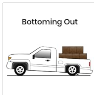
Image 8.1: Diagram showing a truck with a heavy load experiencing 'bottoming out' without proper suspension support.
