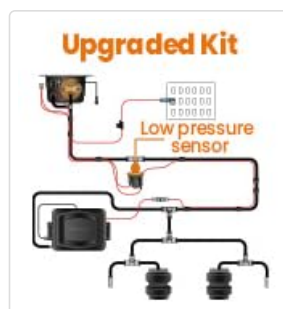
Image 5.2: Diagram illustrating a basic air suspension kit setup with air bags and air lines.
