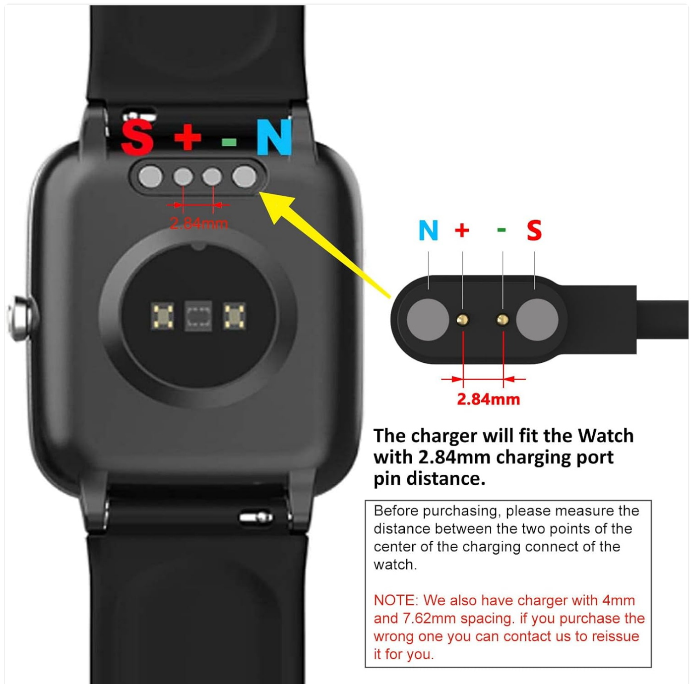
Figure 2.1: Smartwatch charging pin spacing measurement (Note: Image shows 2.84mm, but product is 2.54mm compatible. Please verify your watch's specific spacing).
