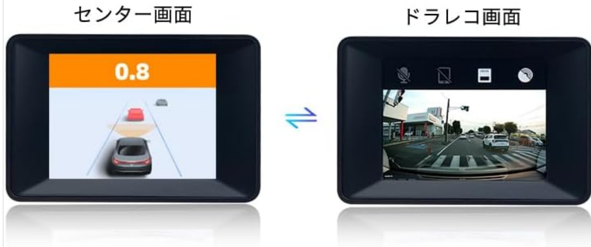
Image 4.1: Illustration of switching between the ADAS center screen view and the dash cam recording view by double-clicking the top button.
