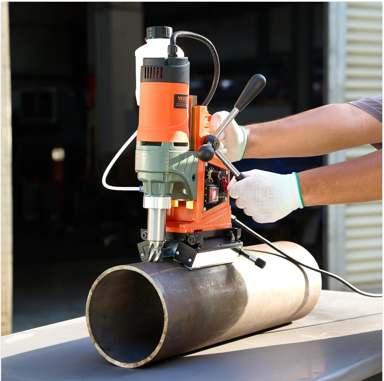
Figure 5.2: Drilling into a metal pipe with the magnetic drill press.
