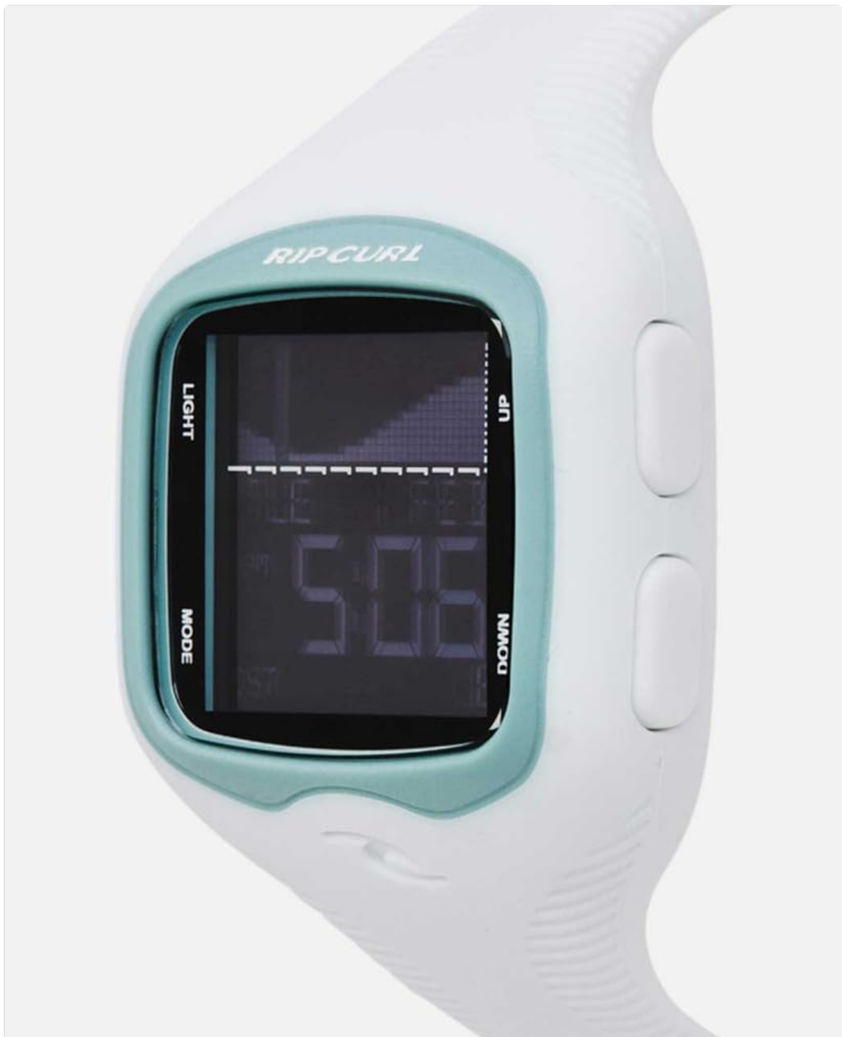
Figure 3: The watch display in Tide Mode, showing a graphical representation of tide movement over time.
