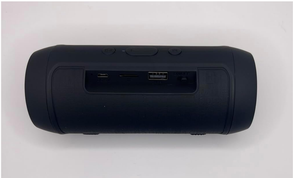
Image: The rear panel of the CHARGE MINI speaker, displaying the DC 5V charging port, TF card slot, USB port, and ON/OFF switch.
