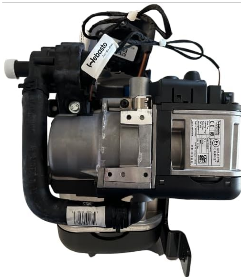
Figure 3.2: Webasto Thermo Top Evo heater with coolant connections, ready for integration into the vehicle's cooling system.
