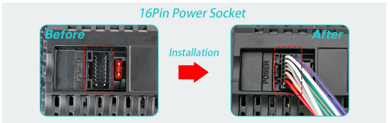
Figure 4: Illustration of the 16-pin ISO connector and its installation into the car stereo's power socket, showing before and after views.
