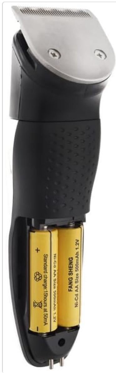
Image 4.1: Bottom view of the trimmer showing the open battery compartment with two AA batteries inserted.
