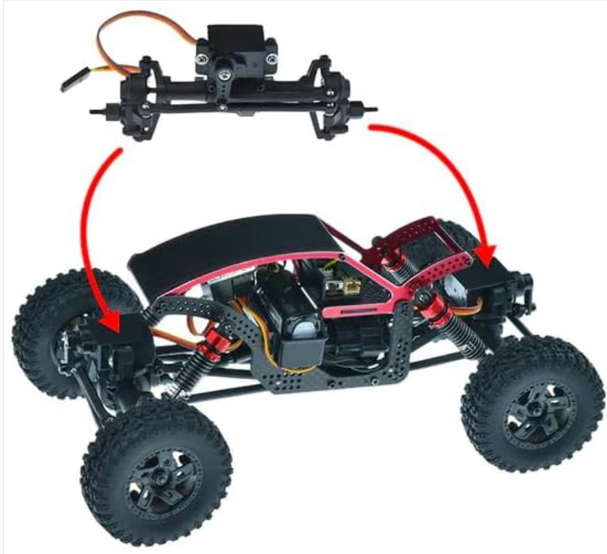
Figure 3: Illustration of the front axle being mounted onto an RC vehicle chassis.
