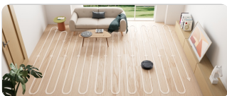
Image: Visual representation of the robot vacuum's zig-zag cleaning pattern for efficient coverage.
