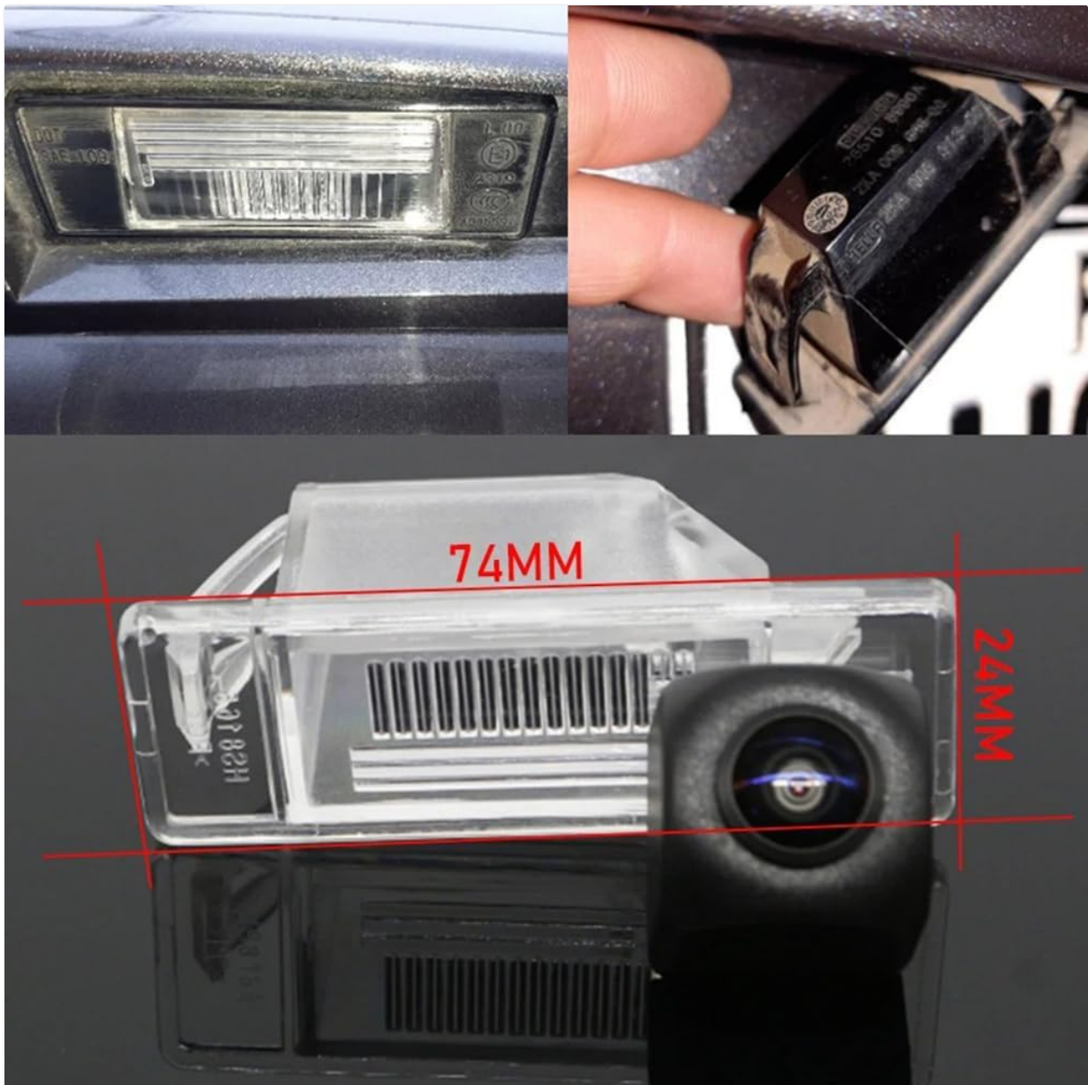
Image: Illustrates the process of replacing the original license plate light with the integrated rearview camera unit.
