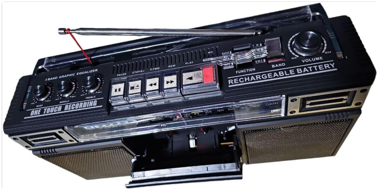
Figure 4.2: Detailed view of the top panel, illustrating the 3-band graphic equalizer (Bass, Middle, Treble), cassette player controls (Pause, Stop/Eject, F.FWD, REW, Play, Record), function selector, band selector, volume control, and tuning knob.
