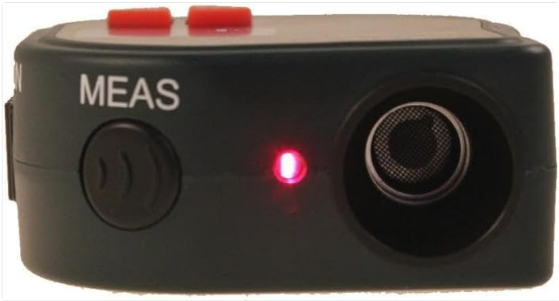
Figure 3: Front view with ultrasonic sensor and indicator light.
